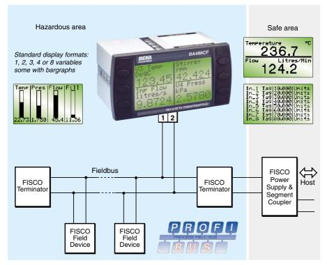
The BA488CF-P Fieldbus Display is an intrinsically safe instrument that can display up to eight fieldbus process variables. Eleven selectable standard screen formats contain one, two, three, four or eight variables, with units of measurement, tag descriptions and bargraphs on some screens.
